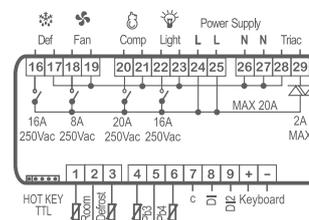
**XW90L** | Digital controller for NT and LT with electrical or hot gas defrost function, fans, auxiliary relay and sixth relay configurable
