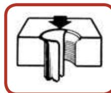
**FORMS STRONGER FLARES-** Stronger flares assured by smooth, even radius formed at base of every flare by engineered chamfer.
