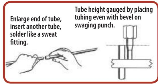
Enlarge end of tube, insert another tube, solder like a sweat fitting.
