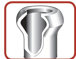
**METRIC BUBBLE FLARING -** Just insert tube flush with top of die for accurate flare. With proper adapter size attached, screw down flaring cone until adapter strikes flaring bar surface. Bubble flare is complete.
