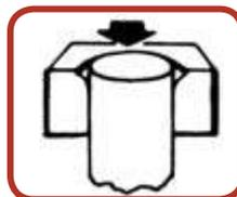
**SELF GAUGING-** Just insert tube flush with top of die for accurate flare size.
