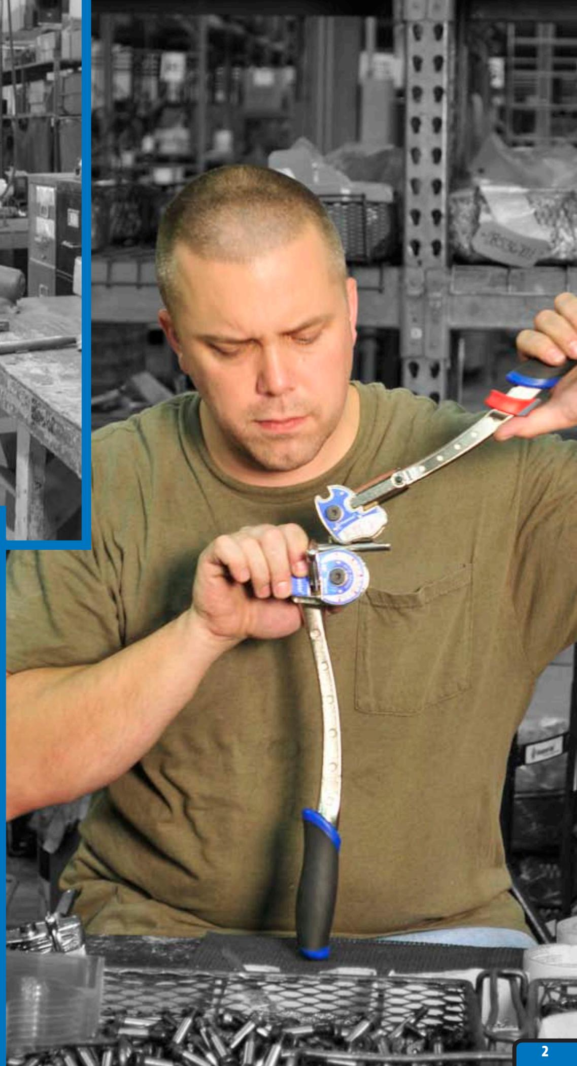
For hard or soft copper, aluminum, brass, thin wall steel, stainless steel, monel, titanium and other tubing.
