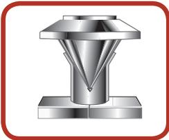
3 rollers in flaring cone. Flare formed above die block.
